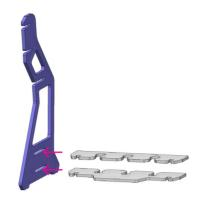
Begin by inserting one end of Shelf 1 through the bottom slot of Side Panel 1, followed by Shelf 2 in the slot above. Ensure both shelves click into place.
