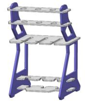
Insert Shelf 4 and Shelf 5 into the top two slots. Once all the shelves are secured, the rack is ready for use.
